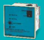
Autoswitch with dry run protection. Auto reset for phase failure faults & manual reset for dry run. Auto/Manual switch. 1 CO output contact. 20 Amps. inbuilt CT, Indications Relay ON Green, Dry run Red, Pre-wired terminals for easy connections
